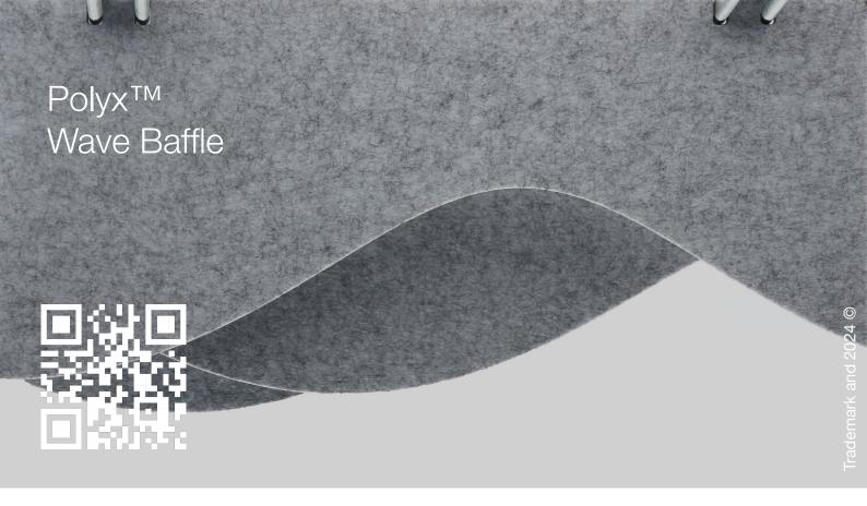
Polyx™ Wave Baffle is a series of undulating baffles inspired by ocean waves. These baffles are slotted into Unistrut channels, for ease of installation. The polyester product is made by a process of tumbling, needle punching, and baking low and high melting point polyester fibres. The high density fibrous network absorbs sounds and reduces reverberation.
