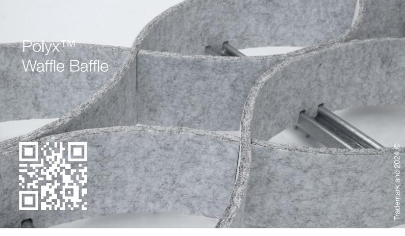
Polyx™ Waffle Baffle is a series of meandering baffles connected together via the waffling method. These baffles are slotted into Unistrut channels, for ease of installation. Polyester Board is made by a process of tumbling, needle punching, and baking low and high melting point polyester fibres. The high density fibrous network absorbs sounds and reduces reverberation.
