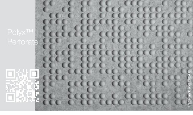
Polyx™ Perforate is created with a network of high-density perforations simulating a binary amplitude diffuser. The panel edges are half-perforated to allow a borderless joinery to the adjacent panel. The polyester product is made by a process of tumbling, needle punching, and baking low and high melting point polyester fibres. The high density fibrous network absorbs sounds and reduces reverberation.
