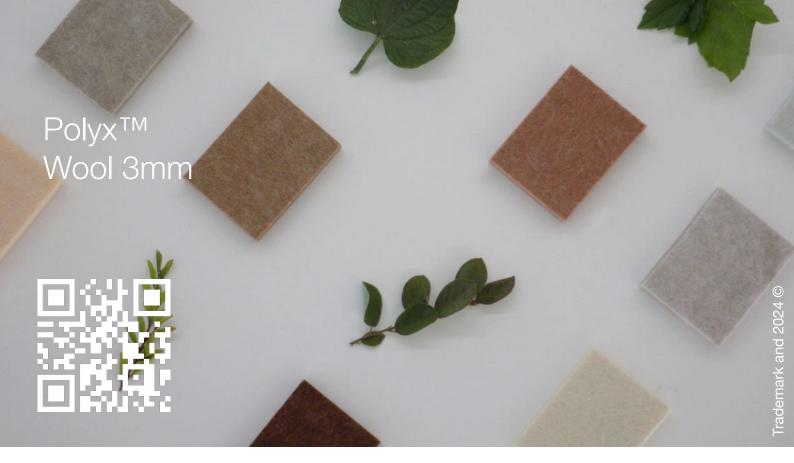
Polyx<sup>™</sup> Polyester Board is made by a process of tumbling, needle punching, and baking low and high melting point polyester fibres. The high density fibrous network absorbs sounds and reduces reverberation. Polyx<sup>™</sup> Board comes in 4 different thicknesses: 3mm, 8mm, 9mm and 12mm.
